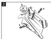
Empty any remaining fuel from original fuel tank. Remove the seat, side panels and radiator scoops. Remove the screws (B) that fixing seat, radiator scoops and tank (G).
