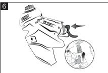
Reconnect the fuel pump power cable and the fuel connector. Assemble the radiator scoops, side panels and seat.
