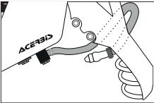
Attach the HUSQVARNA fuel line to the Acerbis tank (A) as indicated in the diagram. Makesure the fuel line isn't folded over, obstructing the fuel flow.
